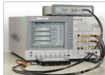
Figure 8. Automated SATA test station
